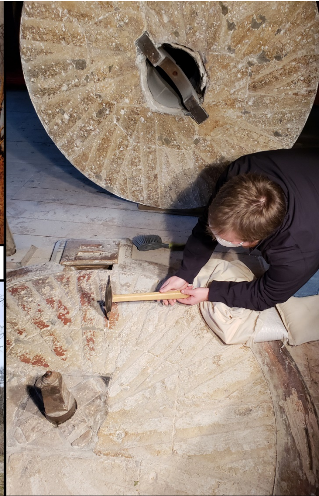
Mill stones being dressed. Source: Scott Foster, November 13, 2018.
